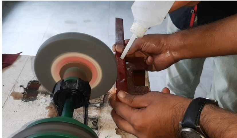
Figure 16: Groove cutting by grinding wheel tool
