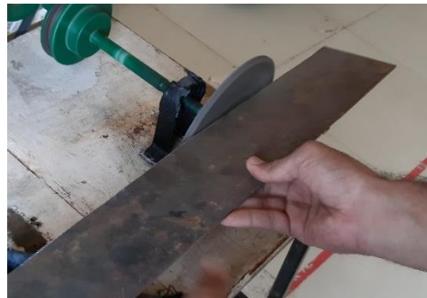
Figure 26: Removing burrs on metal workpiece and prepration of workpiece.
