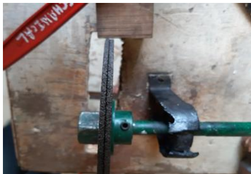
Figure 19: Groove cutting by combination type two cutter
