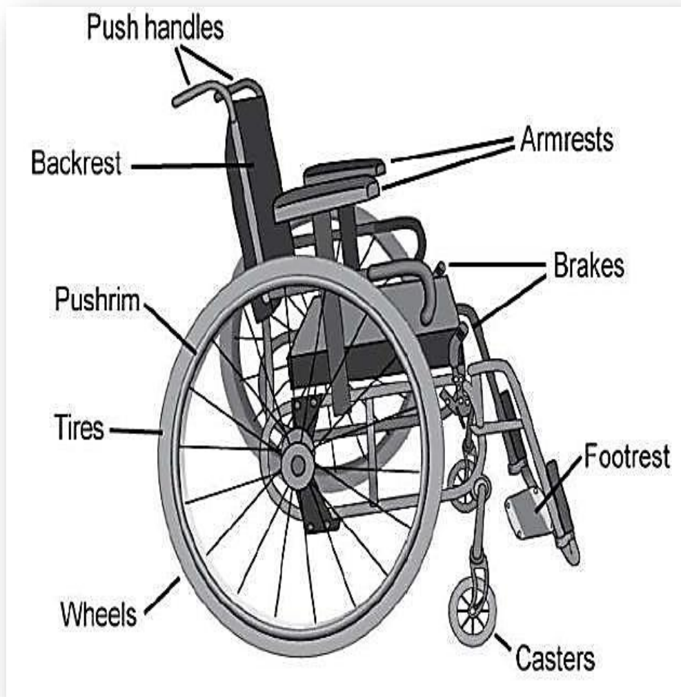
Fig.2.1 Structure of Ordinary Wheelchair
