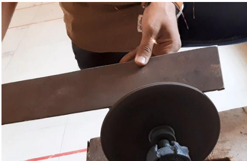
Figure 26: Removing burrs on metal workpiece and prepration of workpiece.
