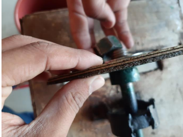
Figure 20: Groove cutting by combination type three cutter
