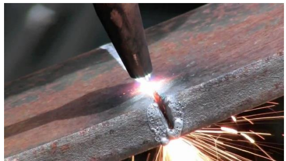
Figure 6(B): Gas grooving method in plate
